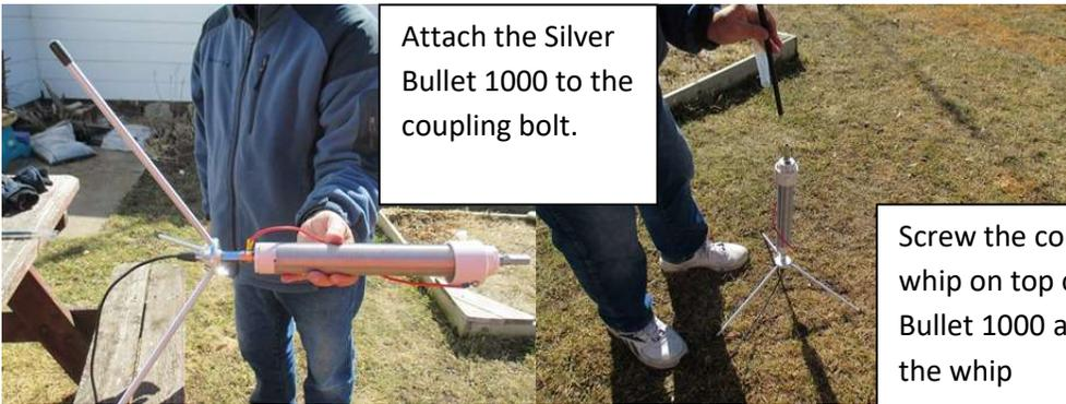
Attach the Silver Bullet 1000 to the coupling bolt.
