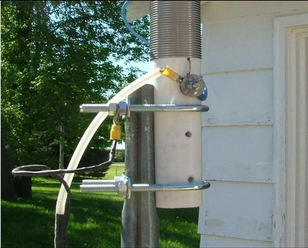
Using common U Bolts the coil can be mounted on a standard TV antenna mast pipe. Attached the braid (ground) side of the coax to the U bolt and the center conductor to the coil input
