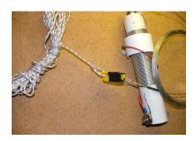
Lastly attach a support to the antenna insulator to a support that can elevate the antenna (like a tree limb). For attic installation you can attach string or other non-conductive support to mount the coil and wire.
