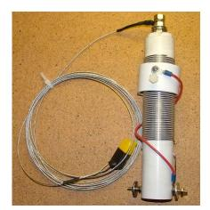
Simply attached the antenna wire to the top of the coil by removing the 5/8 nut slipping the antenna terminal ring over the 5/8 stud and replacing the 5/8 nut. You can hand tighten for portable operation.
