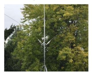
The tuning process stated here is with 102" stainless steel whips. Tuning will vary using longer or shorter whips. Tuning the Otophone is like tuning our Silver Bullet Mini. The difference is you have two coils in a dipole configuration. Put the collars about the same on both coils.
