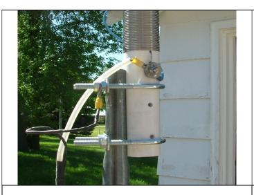
Using common U Bolts the coil can be mounted on a standard TV antenna mast pipe. Attached the braid (ground) side of the coax to the U bolt and the center conductor to the coil input
