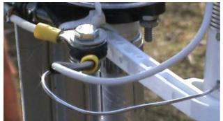
• Cut off excess wire straps and if you want to remove the excess pig tail from the top of the coil.
