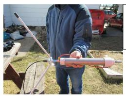
Attach the Silver Bullet 1000 to the coupling bolt.
