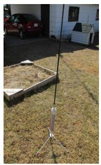
Attach your ground radial and you are ready to tune the antenna. Slide the tuning coupler up and down for max noise on your radio or lowest SWR on your antenna meter. Even with one radial you should achieve a 1.5 or lower SWR on all the bands. For 12, 10 and 6 meters you will need to collapse the whip to get an acceptable SWR.
